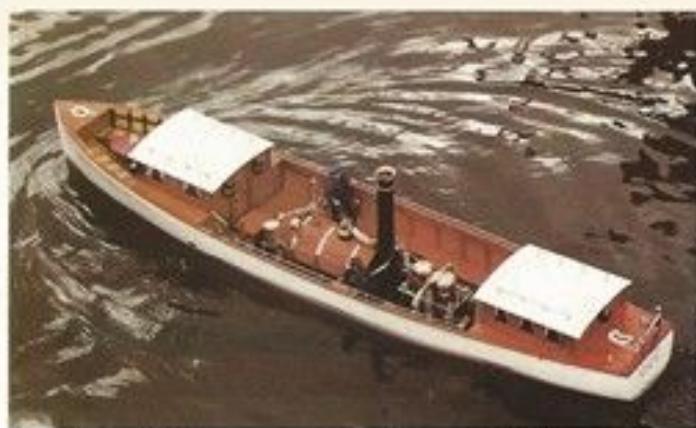
Mary Bell, built by Len Evans, a launch full of character with its timber clad boiler and shining brass work and polished woodwork.
