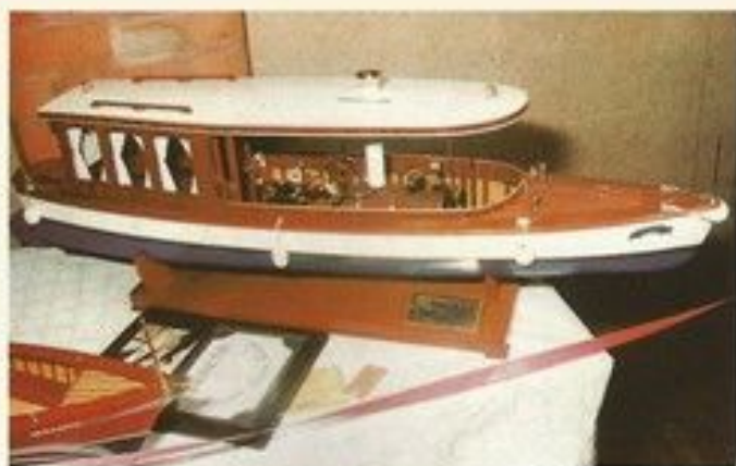
A fine steam launch by E.T. Cook. The hull was moulded in G.R.P.
